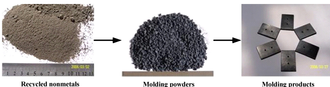
Fig. 16. Schematic illustration of nonmetallic materials of waste PCBs filling in the PMC [7,49].
