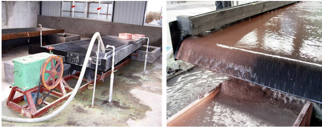
Fig. 7. Fluid bed separation in waste PCBs treatment in Kunshan, Jiangsu province.
