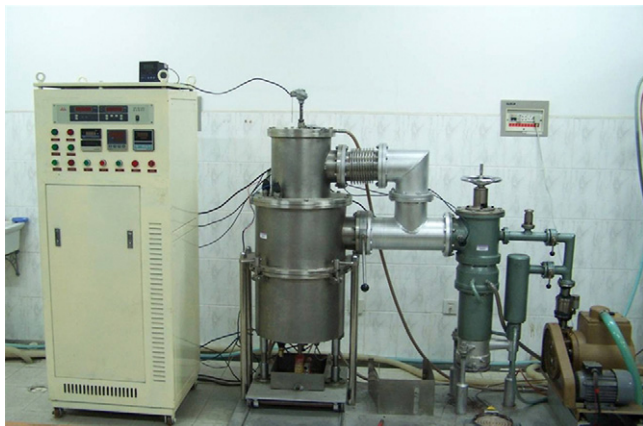
Fig. 15. The vacuum distilling equipment.
